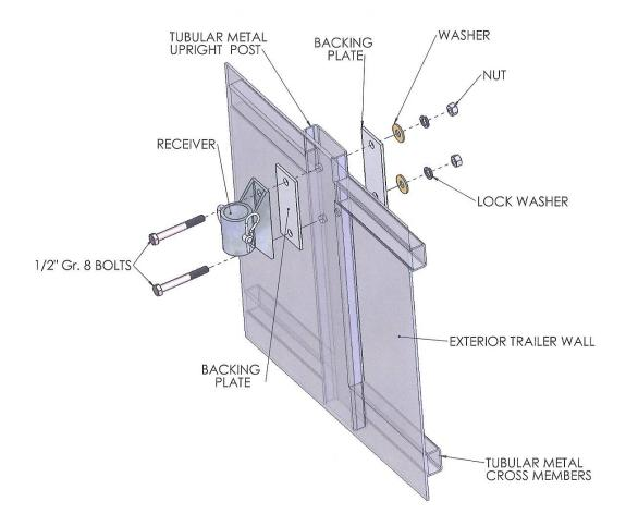
Mount the receiver so that the Spring-Tie <sup>TM</sup> drops in vertically. It is not intended to be mounted horizontally.
